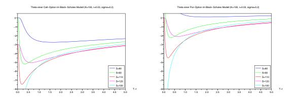
Figure 4.3: Theta of a call (left) and of a put (right). Note that the Theta of a put can become positive for small S.
